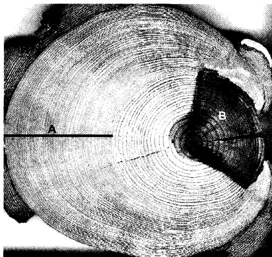
Figure 4. Extent of reaction wood (A) in a ponderosa pine ( Pinus ponderosa Dougl. ex Laws.) caused to lean by floodwaters, Chiricahua Mountains, Arizona. Impact occurred from the right (upstream). Note the compartmentalization (B) (resinosis) behind the impact scar.
